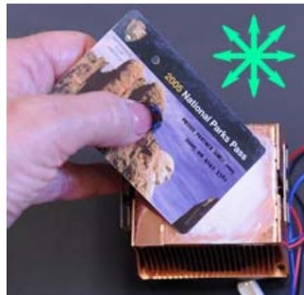
Squeeze enough thermal compound onto the center of this area to create a small mound. By working the plastic tool (old credit card) back and forth in all directions (See green symbol in photo HS1) you will smooth out the compound and work it into heatsink. This will ensure optimum filling of the microscopic valleys in the metal where the CPU cores will contact the heatsink.
